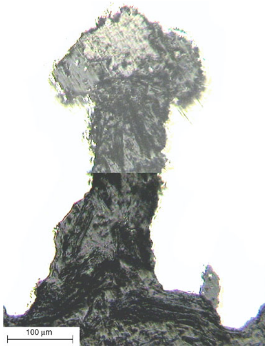
Fig. 9 Photograph of a blunt crack and the blunt crack tip on R-T surface for a specimen cyclically loaded in C2 solution under condition B-1
