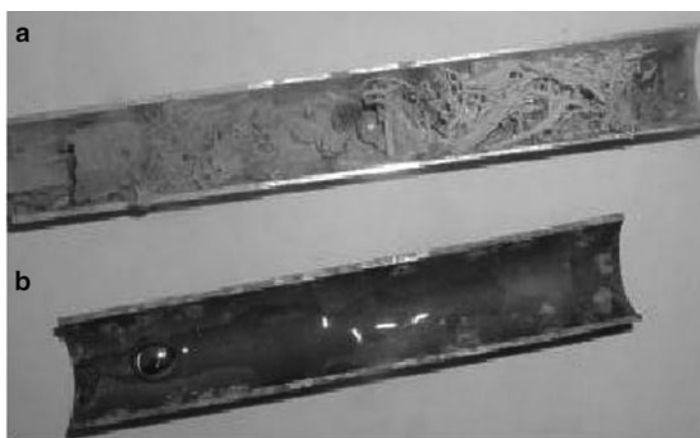
Fig. 9 Comparison between the mercury corrosive attacks of: (a) no coated aluminium tube after 20 min and (b) the coated aluminium tube after 6 month
