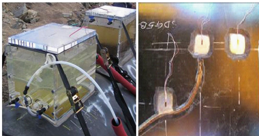
Fig. 1 Samples of in field tests, ( on the left ) in field cells where artificial low pH environment is reproduced and strain gauges on mechanical damage, ( on the right )
