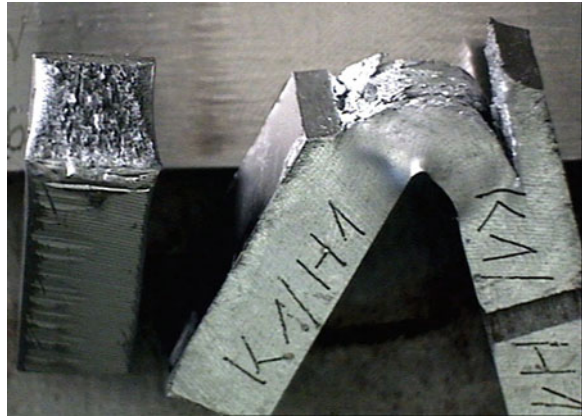
Fig. 3 Typical appearance of the impact tests fracture of specimens cut from (left) the top and (right) bottom parts of the exploited pipe
