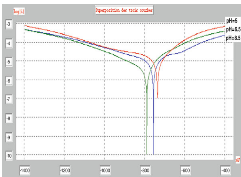
Fig. 1 Potentiodynamic polarization curves of X60 carbon steel in NS 4 simulating solution of corrosive soil environment at 30°C
